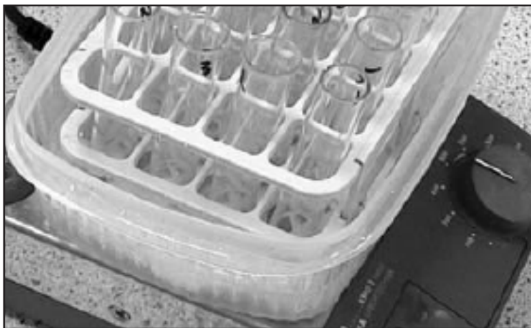
Figure 1. Arrangement of ice-water bath over a magnetic stirrer for dissolution of sample material in 2 N KOH.
