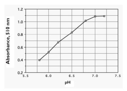
Figure 6. pH Activity curve for B. licheniformis  $\alpha$ -amylase on Amylazyme Red tablets.
