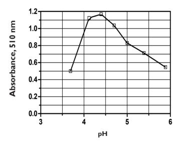
Figure 5. pH Activity curve for A. oryzae  $\alpha$ -amylase on Amylazyme Red tablets.
