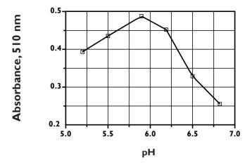
Figure 4. pH Activity curve for malt  $\alpha$ -amylase on Amylazyme Red tablets.
