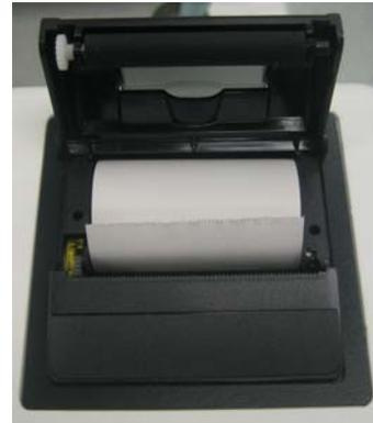
**Figure 1.5.3-2 Printer paper compartment lid open**
